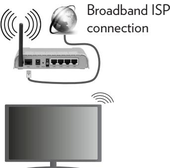
A Wireless-N router (IEEE 802.11a/b/g/n) with simultaneous 2.4 and 5 GHz bands is designed to increase bandwidth. These are optimized for smoother and faster HD video streaming, file transfers and wireless gaming.
