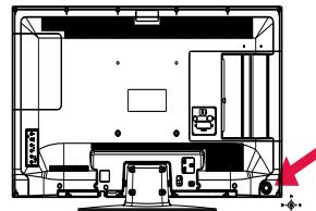
The Control Stick allows you to control the Volume / Programme / Source and Standby-On functions of the TV.
