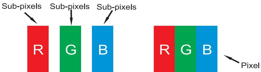
As a requirement of production technologies, the abovementioned sub-pixels may cause "sub-pixel errors" by way of lighting continuously or remaining dim continuously.
